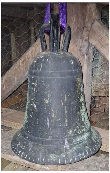
The tierce has six stationary points or nodes around the rim, and two nodes from lip to shoulder. The points of maximum vibration are called antinodes.
